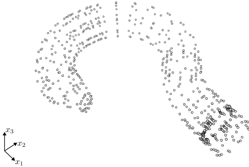
Figure 103 – Collocation points position for the XIGABEM model of hook with crack.
