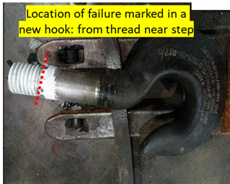
Figure 101 – Fatigue crack location in crane hook experiment (Kishore et al. , 2020).
